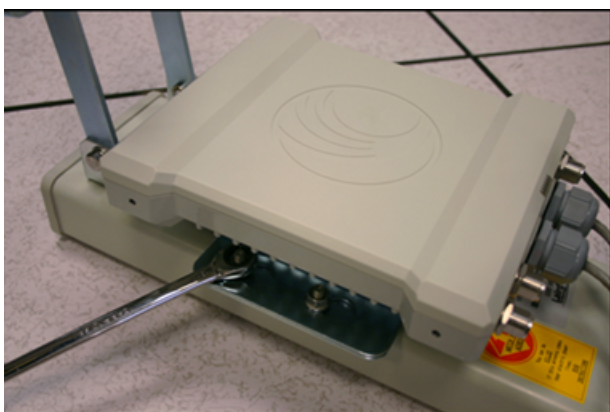
Figure 30: Lower bracket attached to AP antenna
