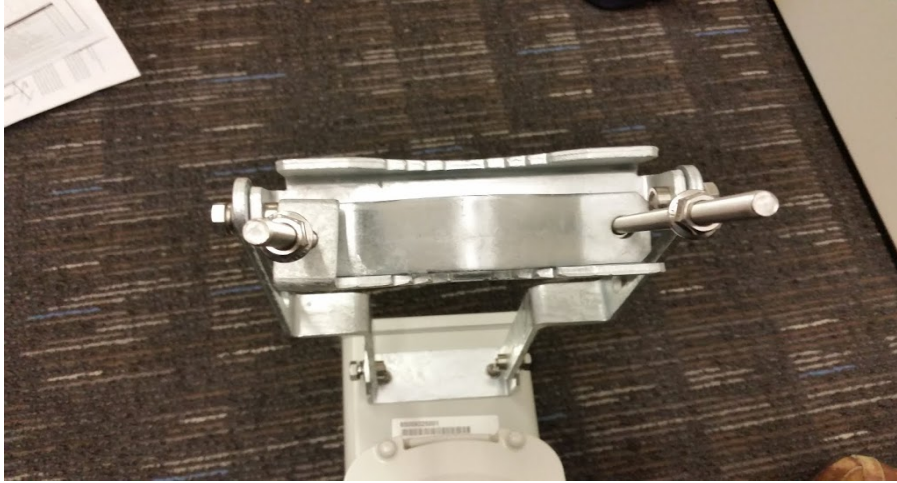
Figure 18: Assembled upper bracket connected to AP antenna
