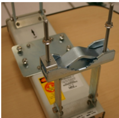
Figure 29: Attaching bracket to the rear of the AP
