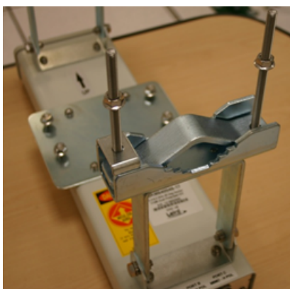
Figure 28: Lower bracket attached to AP antenna
