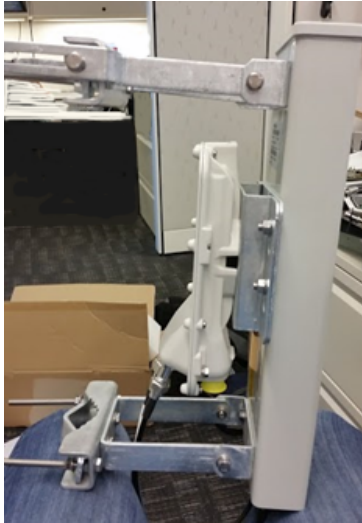
Figure 21: Completed AP and antenna assembly
