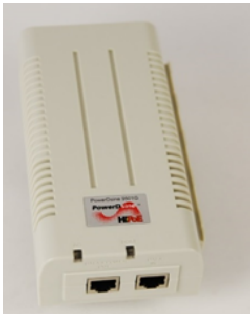
Figure 3: -48 V DC Power Injector interfaces
