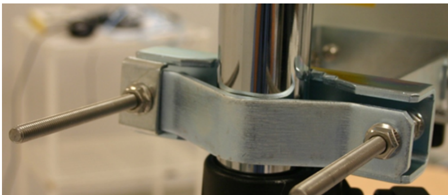
Figure 33: Attaching the AP antenna lower bracket to the pole
