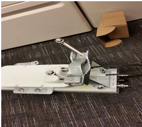
Figure 20: Lower bracket attached to AP antenna
