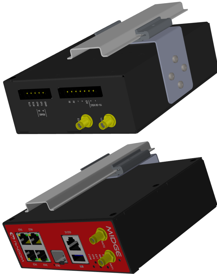
Fig. 4.2: Edged mounting to DIN rail
