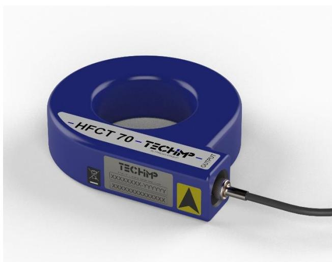
Techimp HFCT 70mm is an inductive sensor for Partial Discharge detection. It is suitable for online/offline PD tests on many electrical systems such as MV/HV cables, transformers, rotating machines and others.
