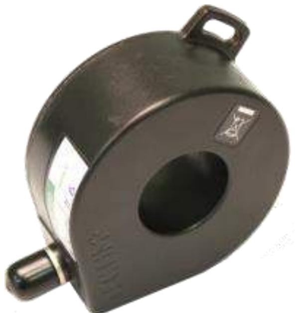
Techimp HFCT is an inductive sensor for partial discharge measurements. It is suitable for on/off line PD tests on many electrical systems (cables, transformers, rotating machine, etc..). It has to be applied to the ground connection of the system to be tested.
