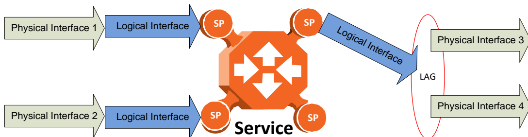
Figure 37: Grouped Interfaces as a Single Logical Interface on Egress Side
