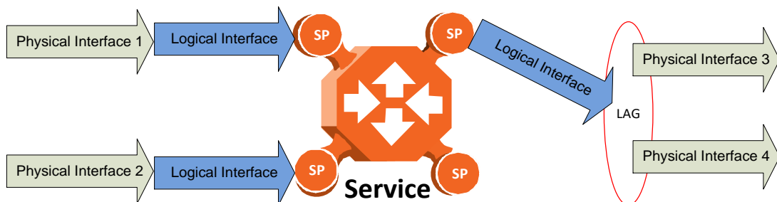
Figure 81: Grouped Interfaces as a Single Logical Interface on Egress Side
