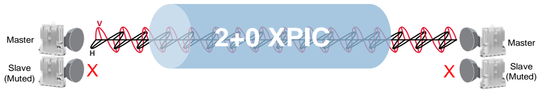
Figure 32: MIMO Resiliency – Master Unit Half-Capacity Link
