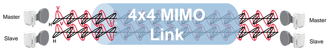
Figure 31: 4x4 MIMO Configuration – Master and Slave Units
