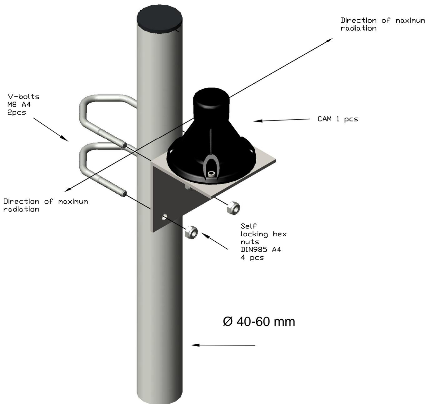
For proper weather protection all connectors and cable junctions should be covered by self-amalgamating tape or equivalent
