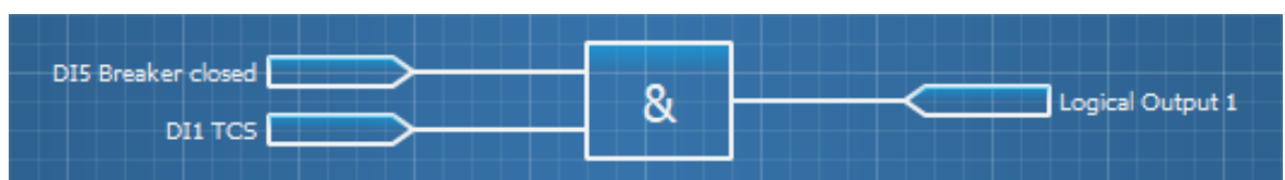
Figure. 6.4 - 187. Example block scheme.
