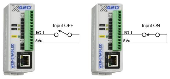
For a low-side switch, one side of the switch is connected to ground and the other to I/O 1 or I/O 2. Select the pull-up resistor. When the switch is open, the pull-up resistor pulls the input high (On).
