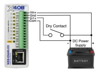
When using modules that are powered using POE (Power Over Ethernet), the 5V output can be used for short wire runs on modules that provide that output. For longer wire runs or for modules that don't provide the 5V output, a separate power supply will be required to "wet" the contacts as shown below.
