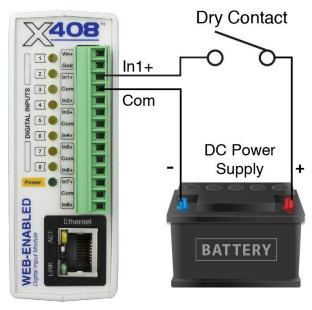
Multiple dry contacts can use the same power supply as shown below.
