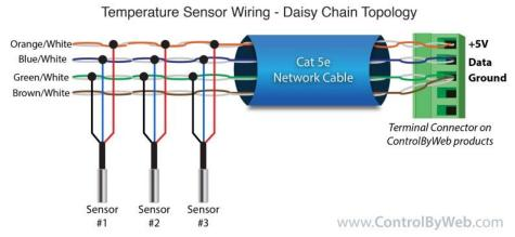
Recommended daisy chain topology connections using Cat5 cable.
