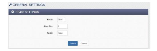
With the X-404 Modbus Master, these settings configure the baud rate, stop bits, and parity of the differential RS-485 bus. The most commonly used configuration is used by default.
