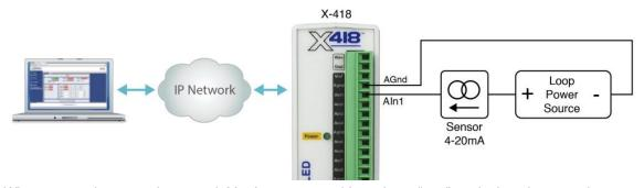
When connecting more than one 4-20mA sensor consider using a "star" or single point ground topology. If the output current from one sensor changes or affects the measurements of other sensors (crosstalk), you will need to re-consider your connections.
