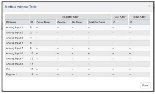
This images shows Modbus address examples for the X-418. Other products tables will differ depending on the device's I/O.
