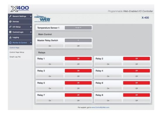
This example shows an X-400 with a temperature sensor, register (named Master Relay Switch), and eight relays that were added from an X-12s expansion module.
