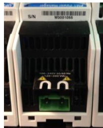
PM1/PM2 rear view - 100~240VAC input terminals
