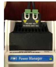
PM1 top view - 100~240VAC input terminals
