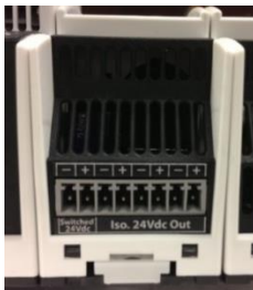
PM2 front view – 24VDC output terminals
