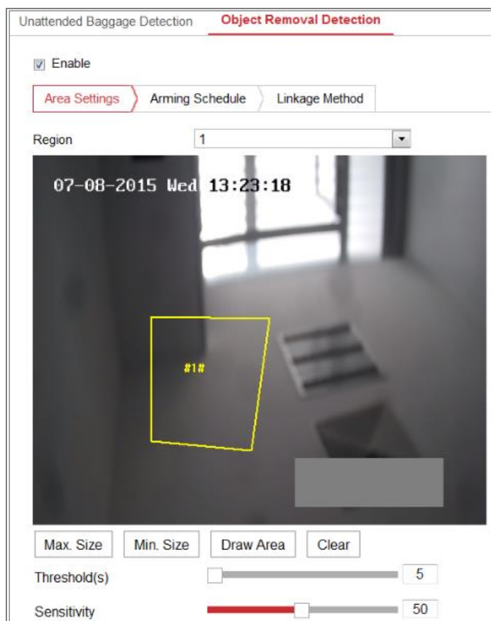
Figure 10-23 Object Removal Detection
