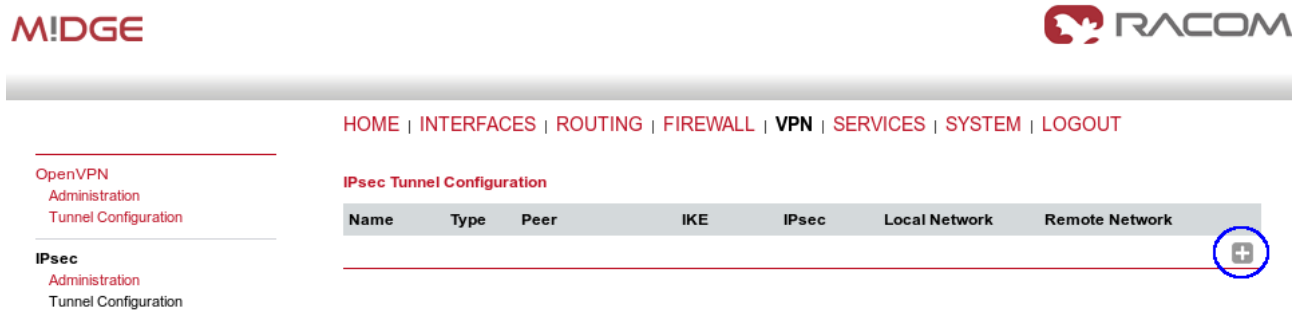
Fig. 2.2: Creating IPsec tunnel
