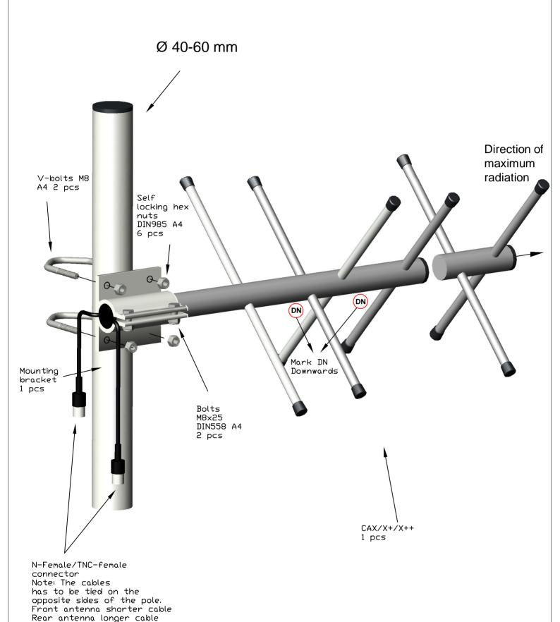
For proper weather protection all connectors and cable junctions should be covered by self-amalgamating tape or equivalent
